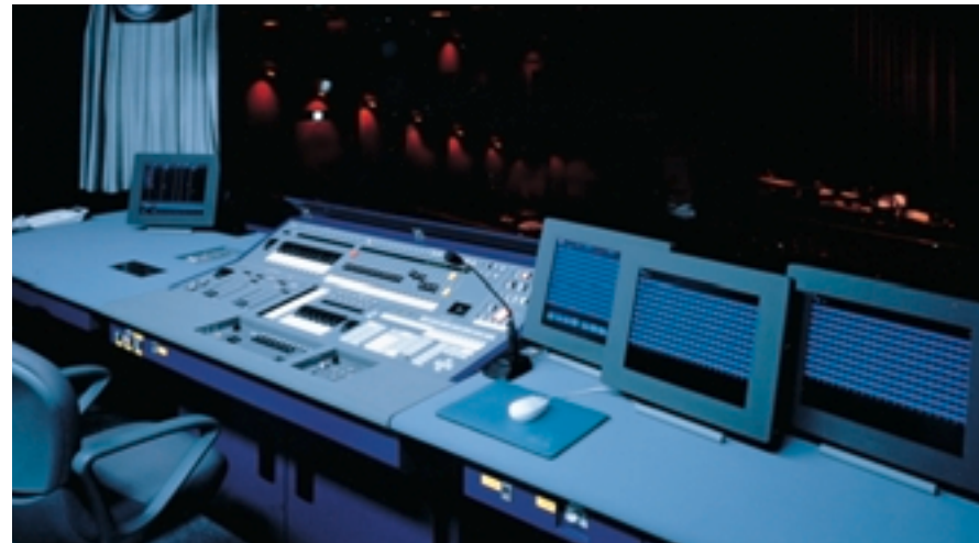
オペラ劇場照明操作卓 A lighting operation console in Opera City Concert Hall
